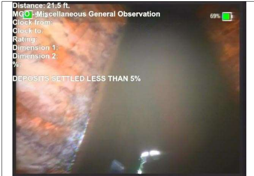
At: 21.5 ft. MGO - Miscellaneous General Observation Joint: No DEPOSITS SETTLED LESS THAN 5%
