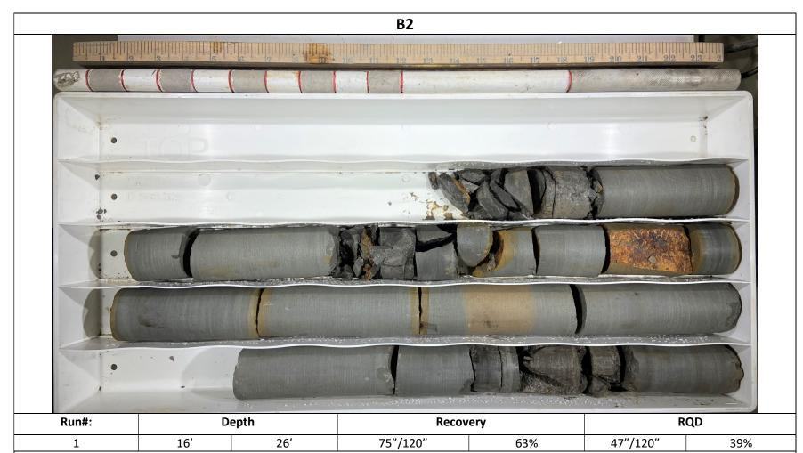
Note: Except for the first two sections, gaps were left at the left end to avoid extra breaks needed to fit core into the core box. Core loss was at the top of the core run in what is believed to have been thinly interbedded very weak, highly weathered, and more intact rock, and is not due to voids in the rock.
