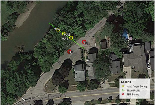
FIGURE 2: Boring locations in the area of the landslide
