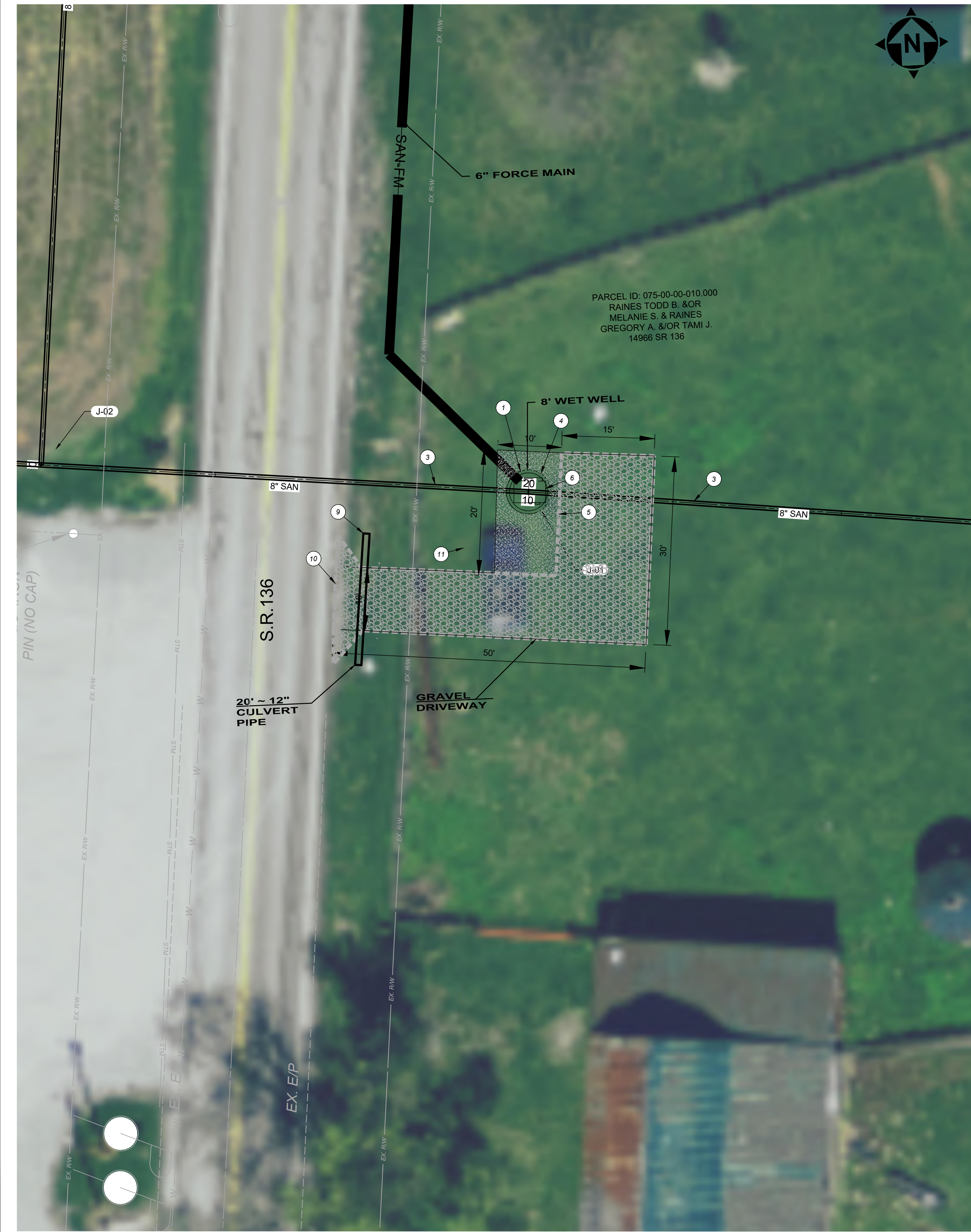
MIDDLE PUMP STATION SITE PLAN SCALE: 1" = 10'
