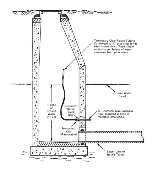
NOTE: Pressurize pipe to 4.5 P.S.I.F. and let stabilize for 5 minutes. Pressure should then be backed off to 4.0 P.S.I.G. and test time started.
