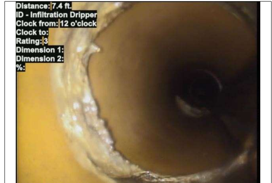
At: 7.4 ft. 12/. ID - Infiltration Dripper Joint: No
