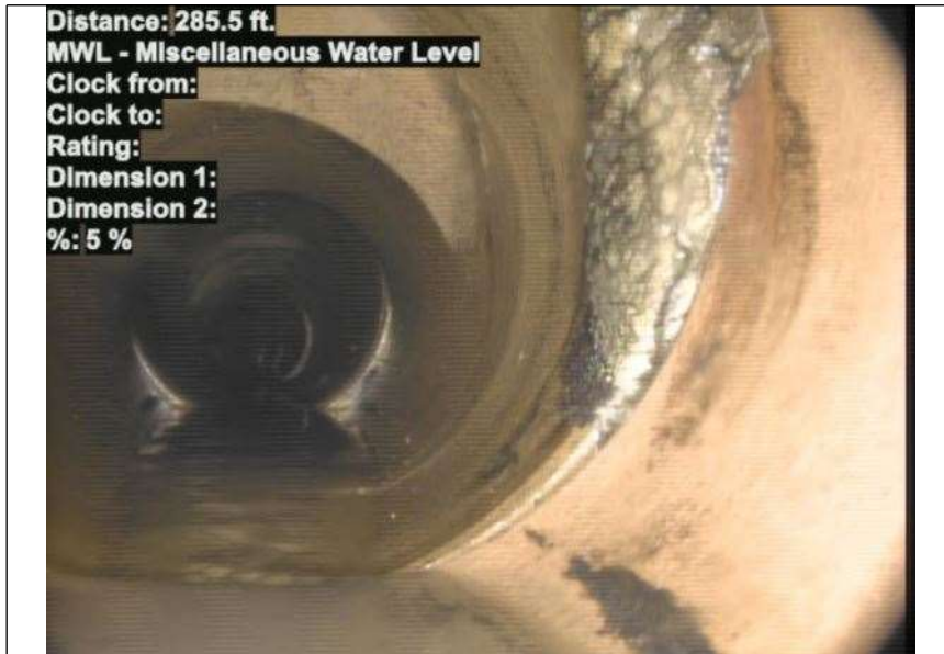
At: 285.5 ft. MWL - Miscellaneous Water Level Joint: No 5 %
