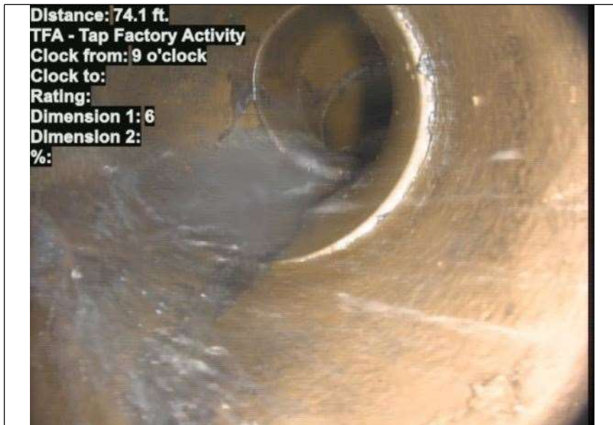
At: 74.1 ft. 9/. TFA - Tap Factory Activity Joint: No
