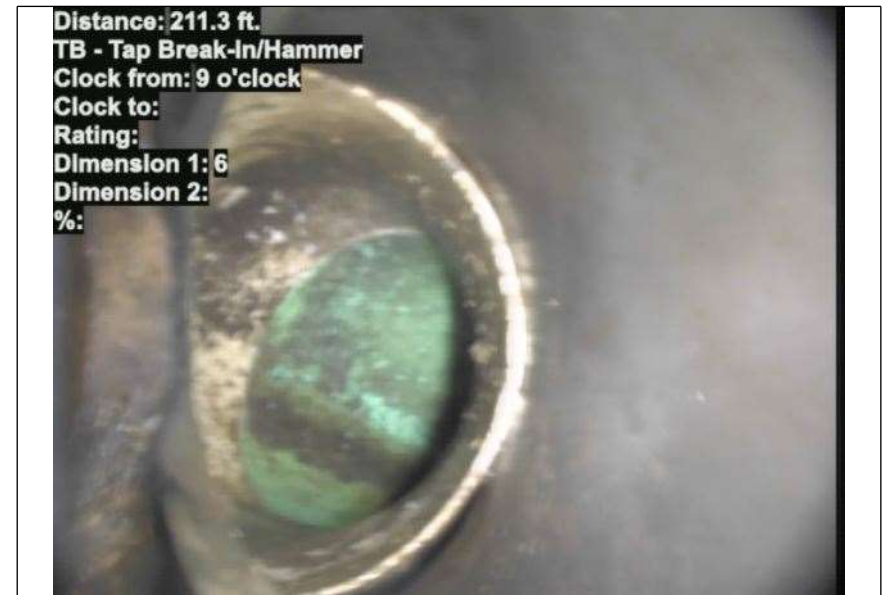
At: 211.3 ft. 9/. TB - Tap Break-in/Hammer Joint: No
