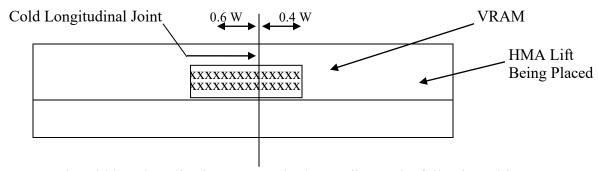
Apply VRAM at the width and application rate required according to the following table:
