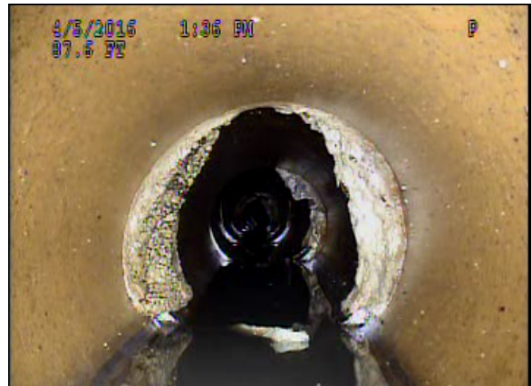
SAS - New Fourth St. – Mineral Deposits at Joints
