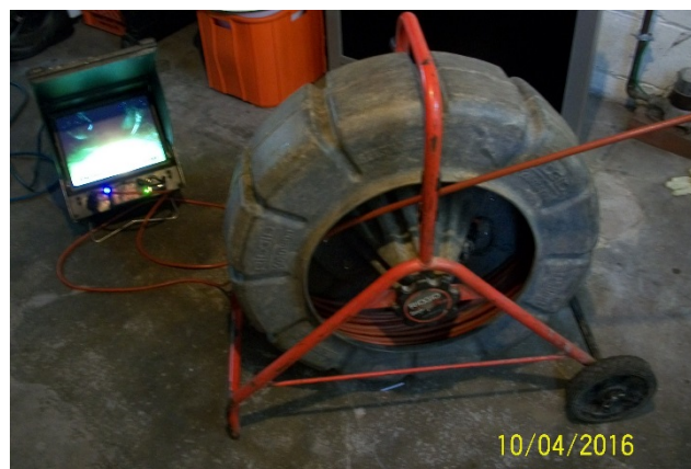
Sewer Lateral Push Camera System
