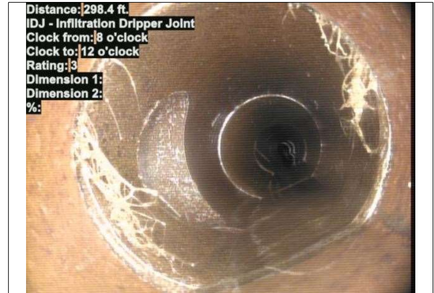
At: 298.4 ft. 8/12 IDJ - Infiltration Dripper Joint Joint: Yes
