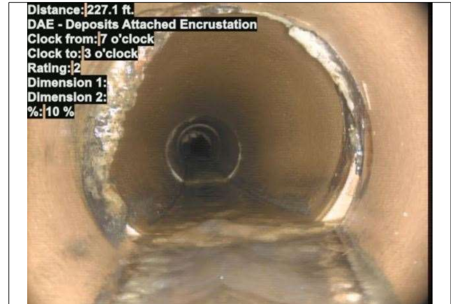
At: 227.1 ft. 7/3 DAE - Deposits Attached Encrustation Joint: No 10 %
