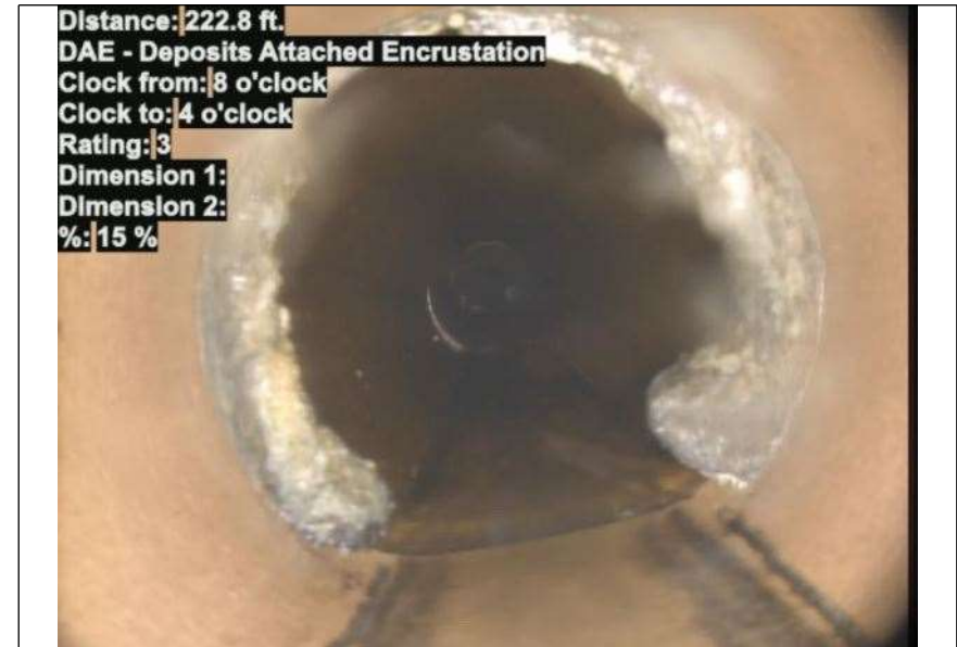
At: 222.8 ft. 8/4 DAE - Deposits Attached Encrustation
