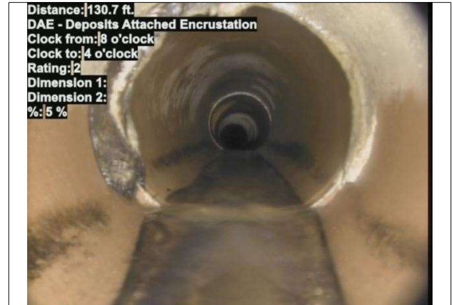
At: 130.7 ft. 8/4 DAE - Deposits Attached Encrustation
