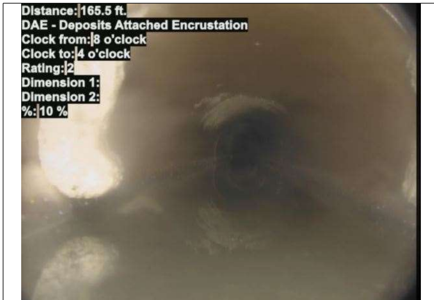
At: 165.5 ft. 8/4 DAE - Deposits Attached Encrustation Joint: No 10 %
