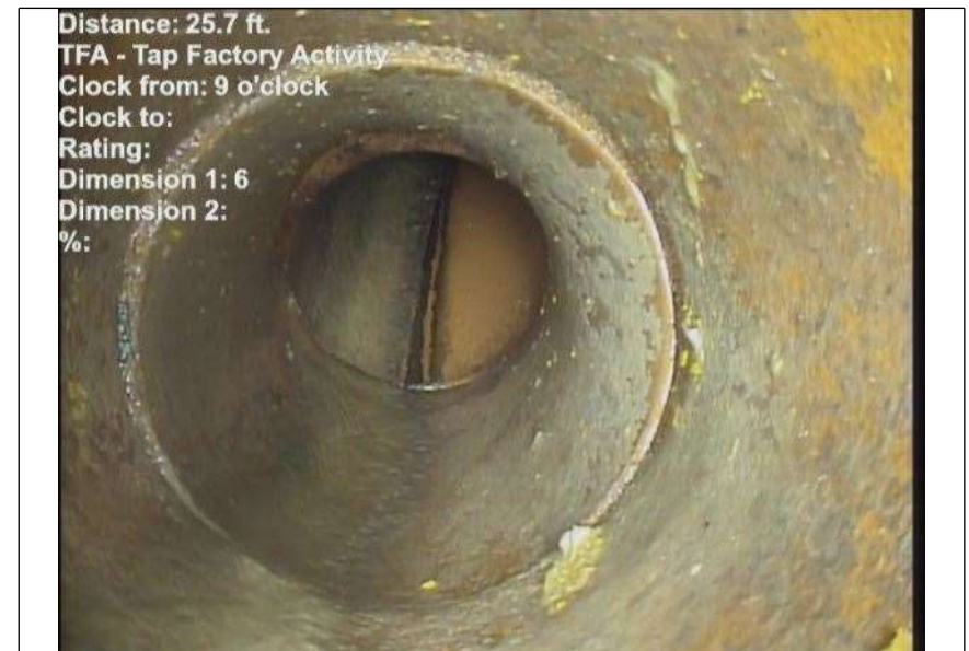
At: 25.7 ft. 9/ TFA - Tap Factory Activity Joint: No
