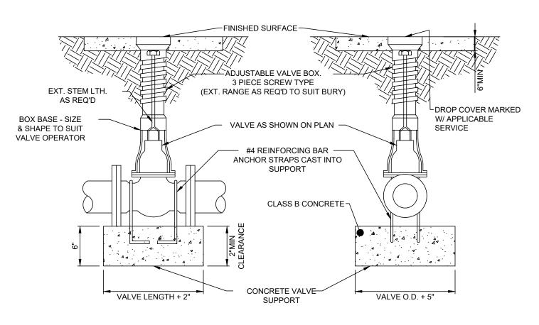
**TYPICAL VALVE AND VALVE BOX SETTING** NOT TO SCALE
