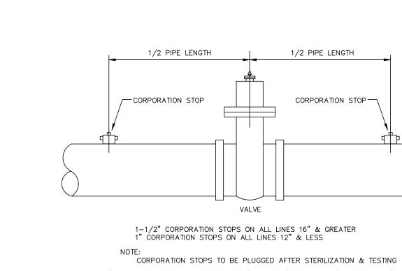
STERILIZATION & TESTING **CONNECTIONS AT VALVES**
