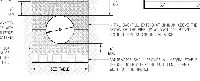
TYPICAL HDPE PIPE TRENCH DETAIL
